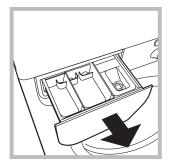
Remove the dispenser by raising it and pulling it out (*see figure*). Wash it under running water; this operation should be
